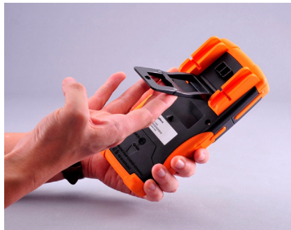
Extend the tilt-stand until its maximum reach
